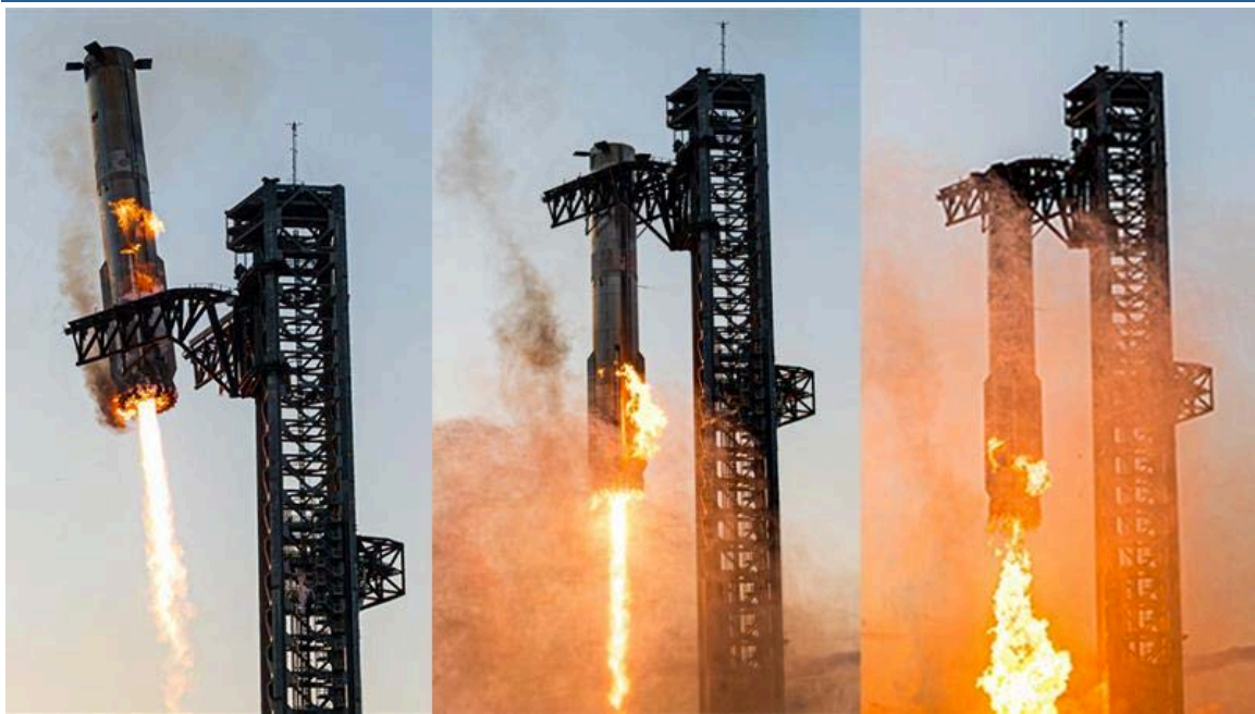
Figure 1. Starship Booster returns to be captured by the ‘Chopstick Arms’ (Credit: SpaceX 1 )
