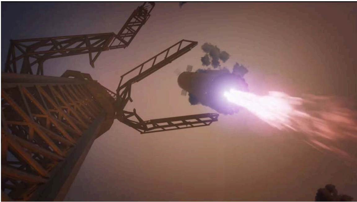
Figure 25. Still from an animation showing a SpaceX Starship Super Heavy booster being caught by the "chopstick" arms of its launch tower after a liftoff (Source: SpaceX 245 )
