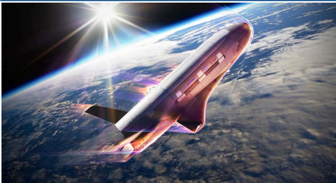
Figure 2. Artist rendering of the X-37B conducting an aerobraking maneuver using the drag of Earth's atmosphere (Credit: Boeing Space 3 )
