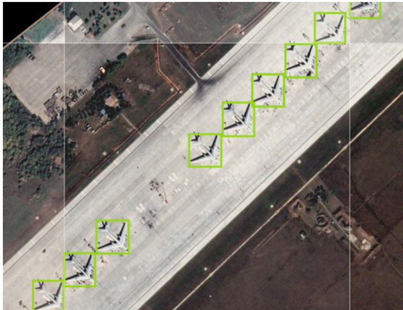
Automated multi-class aircraft detection counted 53,974 aircraft in 1 day from 2,469 scenes and 342 areas of interest. It would normally take a trained analyst 7.5 work days on average to do the same. (Source: Orbital Insight/Airbus)
