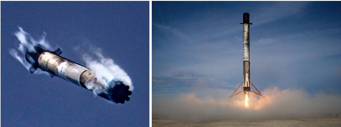
A Falcon 9 reusable first stage during hypersonic reentry and landing at Cape Canaveral, Florida on 25 July 2019. The same core was flown on 4 May 2019 - 82 days prior - and then refurbished. (Source: SpaceX)
